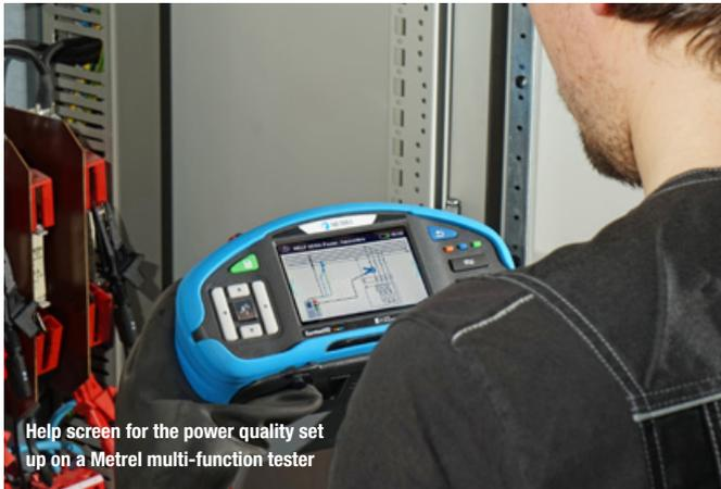
Help screen for the power quality set up on a Metrel multi-function tester
