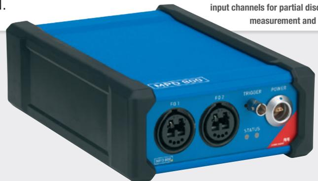
The MPD 800 system can be easily expanded with up to 20 measurement devices connected via daisy chain with fibre optic cables supplied by OMICRON to perform synchronous, multi-channel PD testing at several distributed measurement points. The MPD 800 system software provides users with a convenient overview of all connected devices and the PD measurement data for each measurement channel.
