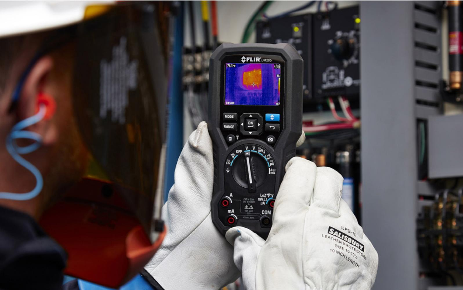
**H**eat is a byproduct of operating any sized electrical circuit. Most problems in electrical systems display themselves in terms of heat. Electricians must be able to classify a circuit as normal when the load is on, or identify when it is abnormal and identify the issues that presents – finding hot spots that need attention.
